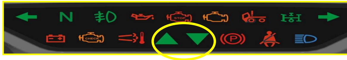
Gear Shift Advisor in Instrument Cluster
